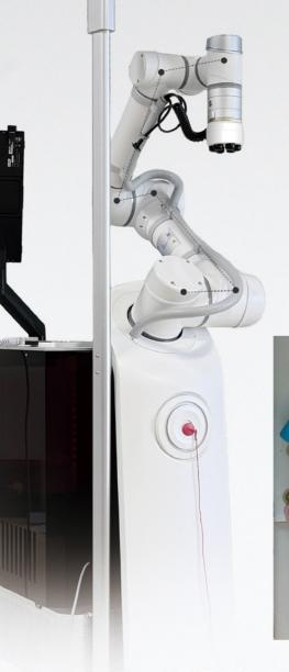
Flexible collaborative robotic arm is based on 6-joint electric drive, and Al image body recognition, pre-programmed movement trajectory, more flexible and precise movement, higher collision avoidance, safety and reliability.
